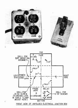
Drill center diagram saves detail measurement for mounting junction box components.
