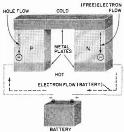
Fig. 6. Pictured here is a basic semi-conductor module used in the Carrier Corp. air conditioner. P- and N-type semiconductors are used.
