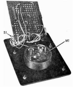
Vectorboard is cut within meter panel dimensions; resistors are positioned for the best fit.
