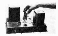
Capacitor sockets permit "filter cans" to be plugged in and taken out like tubes.
