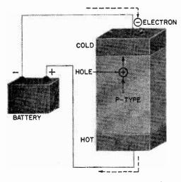
Fig. 5. Not only can electrons move heat from one place to another, so can holes. Incoming electrons combining with holes cool the top metal plate and heat the bottom.
