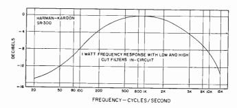
Keeping the output signal at rated output and less than 1% THD at 1000 cps., the amplifier's response varies less than ±1 decibel throughout the wide-band frequency range recorded.
