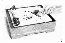
To keep wow, flutter and rumble at minimum a belt drive (held by finger) is used. Stepped pully and idler permit the speed selection.
