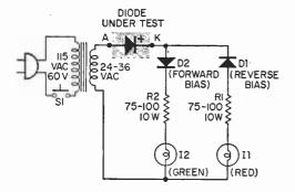
Build It Now. Why not have a diode tester on your workbench now so it's ready to hunt down a culprit diode before your battery needs charging. This one's a simple, easy to use, inexpensive device that will test for open, shorted, or even leaky diodes. Its indications are easily interpreted to obtain the condition of the alternator diodes, or other diodes used in radio, television and battery chargers for example.
