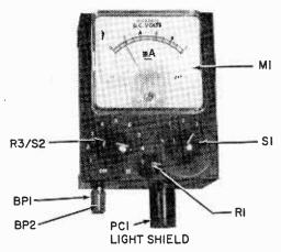
Design-for-function quality of the flashlight tester makes it easy to work with.
