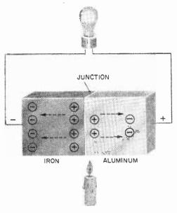
Fig. 2. Diagram shows how heat creates thermoelectricity—the famous Seebeck effect.
