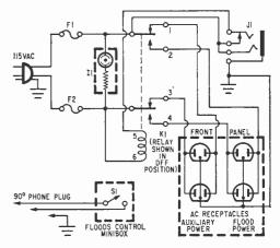
Schematic diagram of the control unit indicates function of relay K1 in circuit.
