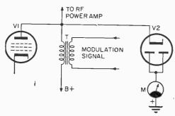
The over-modulation indicator shown can be used with a CB set or low power ham rig. Tube V2 is a 6X4 or dual diode, or it can be semiconductor diodes. The meter may be a DC voltmeter or a 0-1 DC milliammeter. The primary of transformer T is the modulation reactor. The meter needle will "kick" when the modulation exceeds 100% at which time the voltage to the RF amplifier is actually negative instead of positive.
