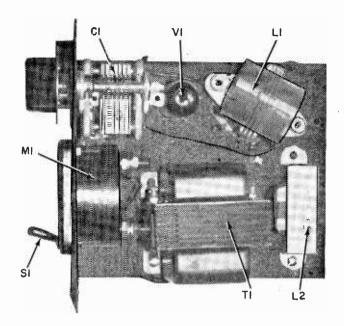
Operation was restricted to mainly 160, 80, 40, and 20 meters. For operation on 20 and 15 meters it is advisable to reduce the value of the pi-network capacitance by taking capacitor C9 out of the circuit.
