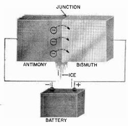
Fig. 3. Pictorial diagram showing the Peltier effect—as electrons cross junction of dissimilar metals, the antimony-bismuth junction is cooled.
