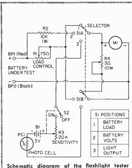
shows switching circuits for the two tests.
