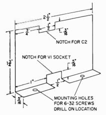
Detail drawing of the copper shield partition installed inside the VHF Extender. Dimensions may vary slightly depending upon how accurately Nuvistor socket is placed.
