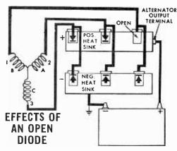
Open diode will not let current flow in either direction. The circuit is not complete through the B winding to battery.
