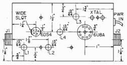
Detail drawing of chassis top part's layout.
