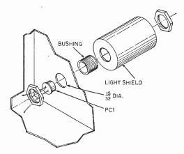
Light-tight use of bushing and shield in detail drawing of photocell installation.
