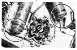
Another sure trouble spot (inside circles), paper coupling capacitors with wax oozing out of the cases. It is wise to replace with "ageless" moulded types.
