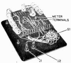
The meter terminal lugs provide convenient mounting points for the wired vectorboard.
