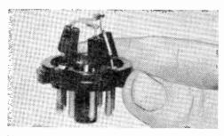
If you want to check whether your amplifier can use silicon diodes in place of the rectifier tube, an adapter can be made by wiring SR's across tube base.
