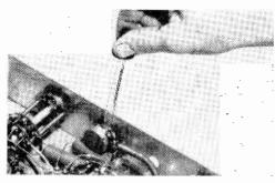
Many noisy tone and volume controls can be silenced with a few drops of "nonoise" squirted into the volume control.
