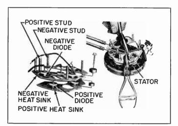
Access to the Autolite alternator diode assembly, described in text, is easy. When soldering or unsoldering diodes always use heat sinks to avoid damaging the diode. Here, pliers function to carry heat away.
