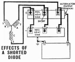
Shorted diode will allow current to flow in both directions. It will flow back to the A winding instead of to the battery.
