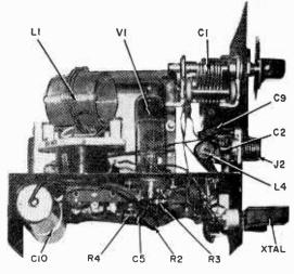
Side view of the transmitter shows placement of parts above and below the sub-chassis.
