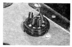
You can either wire the diodes to a plug as the author did or wire them under the chassis directly to the rectifier socket.
