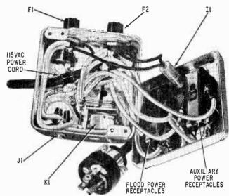
on a tripod leg in the most convenient position for the photographer. It houses FLOOD CONTROL switch S1. The s.p.s.t switch is rated at 5 amperes at 125 volts. The switch shown happens to have a safety cover since it was recruited from a war surplus miscellany box. Three spring clips are mounted on the rear cover of the Minibox to secure it to the tripod; choose size to fit your tripod.
