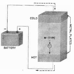
Fig. 4. Semiconductors do a much better job than metals in cooling a junction. Like Robin Hood, electrons take excess heat from the top plate and transfer it to the bottom plate.
