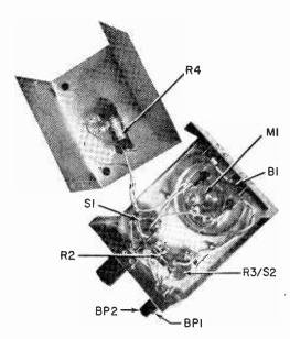
Aluminum chassis box (3"x4"x5") provides good spacing for all the tester components.
