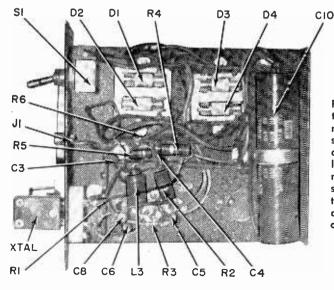
Front panel of one-tube five-watter is shown above. Key is connected to jack J1. Underside of sub-chassis, left, is not wired with components held to a specific location; but, in general, keep the radio frequency wiring near the side of the chassis (bottom of photograph). Power supply wiring, diodes and holders are visible on other side.
