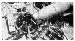
To simplify future repairs and tests, capacitor sockets are substituted for mounting wafers. Note that components are connected to lugs like on tube sockets.
