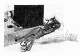
First thing to do is replace old power cord if it shows cracks. While you are at it, make it extra long. Add fuse holder if set has no overload power line protection.
