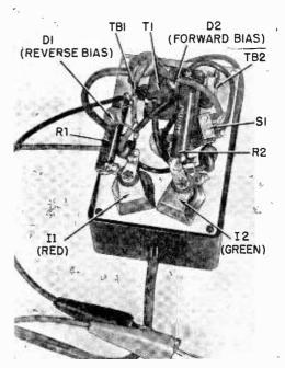
Rear view of meter case panel shows placement of parts. Test setup, below, shows anode (A) and cathode (K) test leads connected to an alternator diode. Anode is copper wire, cathode is the case of the diode.
